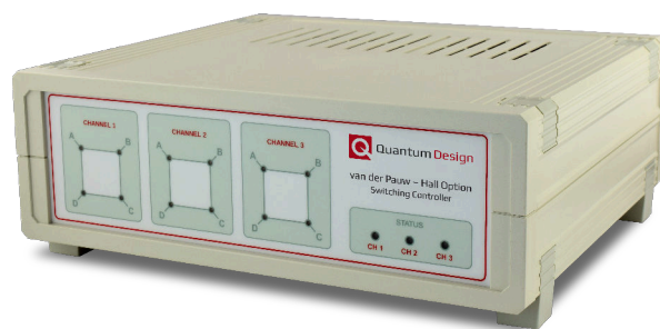
Figure 3: The van der Pauw-Hall Option switching controller automatically performs permutations of the current and voltage leads and collects the data required for calculation of carrier concentration and sheet resistance for a uniformly thick sample of arbitrary shape.
