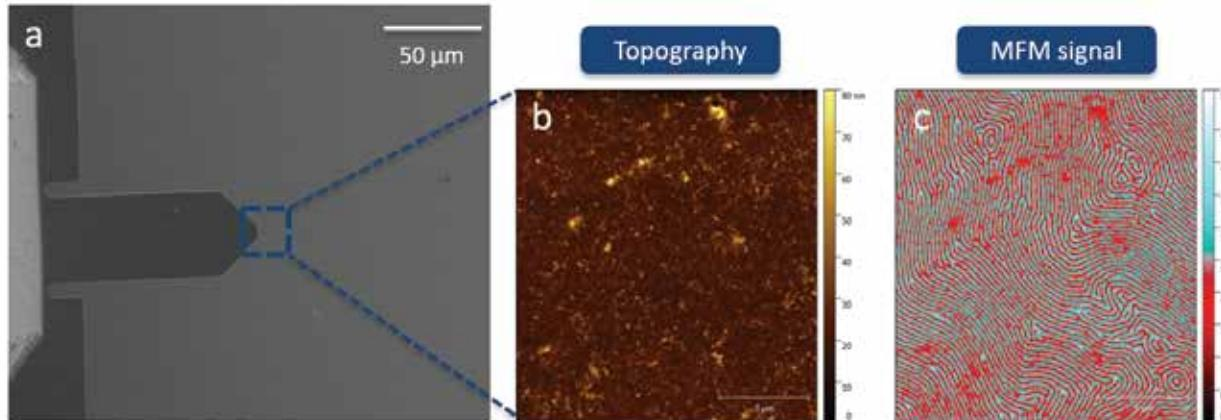
Topography and MFM measurements on a multilayer sample provided by G. Hlavacek, O. Hellwig (HZDR, Germany). SEM guidance allows one to find the region of interest (a); AFM topography image of a smaller area (b); and the corresponding MFM signal measured with magnetic “super-tip” (c).
